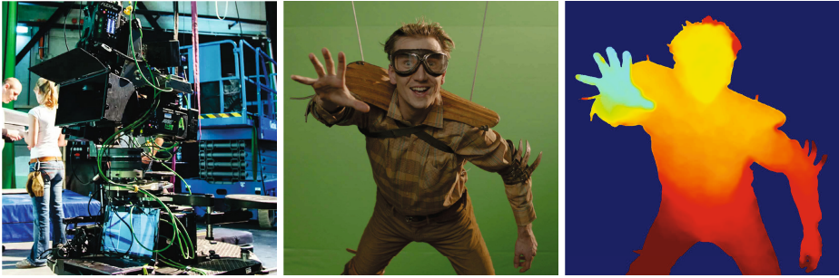
Fig. 1. From left to right: Stereo-ToF rig on set, example image, high resolution disparity map
