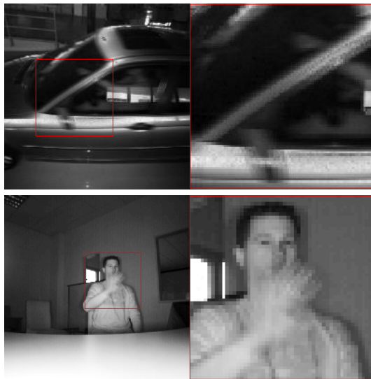
Fig. 2. Top: Demodulation of the car's phase image sequence and a corresponding closeup. Bottom: A moving hand scene and a corresponding closeup. Left: Motion areas are marked red. Right: The closeups of the red marked motion areas.
