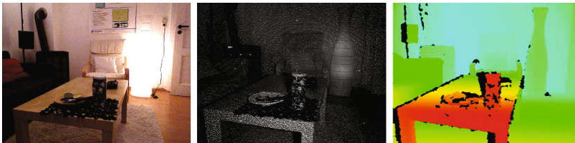
Fig. 2. Typically, the Microsoft Kinect would be found in the living room of a Microsoft Xbox user. Left: typical usage scene, Center: infrared pattern, Right: colorcoded depth map.
