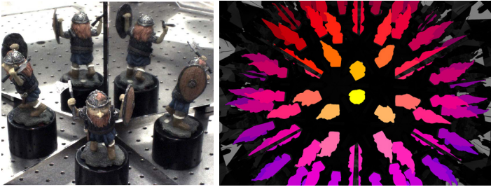
Fig. 17. The five-view case employing inter-reflections up to second order [25] – self-occlusion is clearly visible (left). In the case of many inter-reflections a pixel labeling procedure is necessary [2] that can resolve the view assignment to pixels – up to eight reflection levels have been employed (right).
