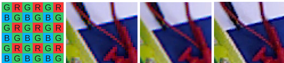
Fig. 6. Left: the Bayer pattern as it is used in the Microsoft Kinect camera. Center left: a Kinect color image converted to RGB with a fast demosaicing method as it is used in the Open NI driver. Center right: demosaicing result by a simple bilinear demosaicing method. Right: demosaicing result by the AHD method as it is implemented in the DC1394 library.
