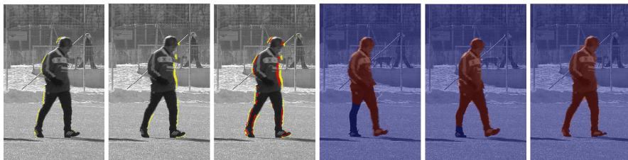
Fig. 2 Occluded regions are regions of one image that back-project onto portions of the scene that are not visible in another image. They can be determined by comparing multiple images of the same scene, and inferred together with the domain deformation w or its linear component (optical flow) by solving a convex variational optimization problem [3].
