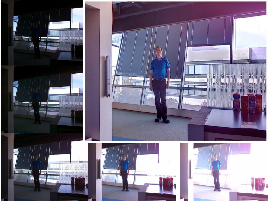
Fig. 5 A burst of five image taken with different exposures (left and bottom) are fused into a single image that shows details both in the bright and dark areas better than in any of the input images.
