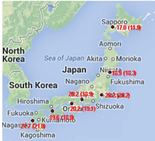
Fig. B.5 Design outdoor humidity ratios in main cities of Japan (unit: g/kg) (Note: Data out of brackets is parameter for no assurance of 0.4 % and in brackets is 1.0 %)
