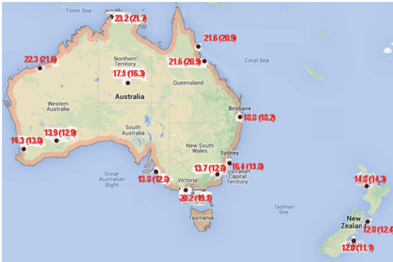
Fig. B.4 Design outdoor humidity ratios in main cities of Australia and New Zealand (unit: g/kg) (Note: Data out of brackets is parameter for no assurance of 0.4 % and in brackets is 1.0 %)
