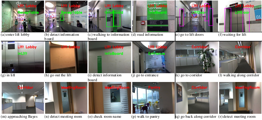
Fig. 3. Typical navigation sequence for a visitor headed to meeting room Bayes on the 10th floor. In each example image, the red text superimposed on the image indicates the recognized scene, the green text indicates the recognized location, the green box indicates the detected information board, and the pink box indicates detected lift doors.
