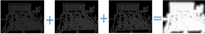
Fig. 2. The weight map is generated by the summation of dilated edge maps
