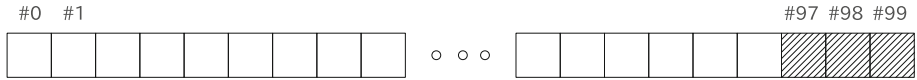
Fig. 1. A one-dimensional cable of the FitzHugh-Nagumo models. The cable consists of 100 FHN elements. The right 3 elements are periodically fired by a constant depolarizing bias current. The left 10 elements are stimulated by a short depolarizing pulse.
