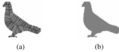
Fig. 18. Shape reconstruction from the MA: (a) Original shape and its MA; (b) The shape reconstructed from the MA [47]
