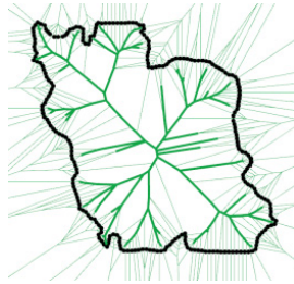
Fig. 11. The MA is a subset of the Voronoi edges
