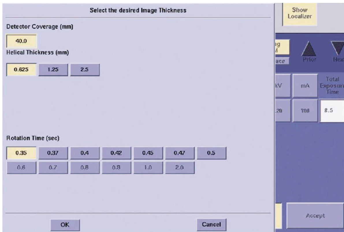
■ Fig. 9d.6 For cardiac scanning, choose the detector coverage, helical thickness, and rotation time as shown in this screenshot
