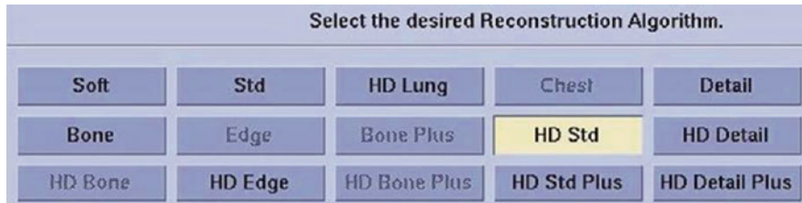
Fig. 9d.13 Choosing the cardiac scan type and the high-resolution option, the user can select the “HD Std” kernel or the “HD Detail” kernel. HD Detail allows having higher spatial resolution but is also noisier than HD Std and may thus be best suited for stent analysis and heavily calcified vessels
