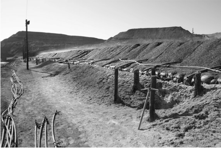
Fig. 7.4 Leach pile or heap operation (acid leach) for high-grade copper oxide ores
