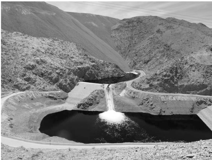
Fig. 7.6 Collection facility for PLS of a mayor (bio) leaching operation. After SX-EW, the solution is recycled to the leaching process
