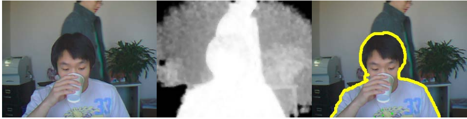
Fig. 1. Example segmentation result by fusing color and depth information using Dempster’s theory of evidence. The explicit modeling of uncertainty forces the algorithm to segment the person in the foreground even if the depth information of the person in the background is similar. Input data taken from [9].
