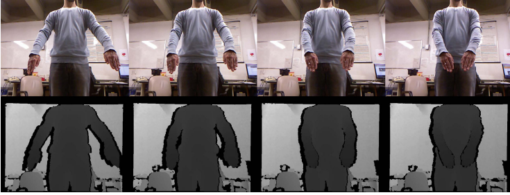
Fig. 1. Input data is a video sequence of texture and depth map images per frame, providing the RGB and (x, y, z) values of each pixel
