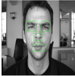
Fig. 1. One training image from the BioID database with the four proposed face parts shown
