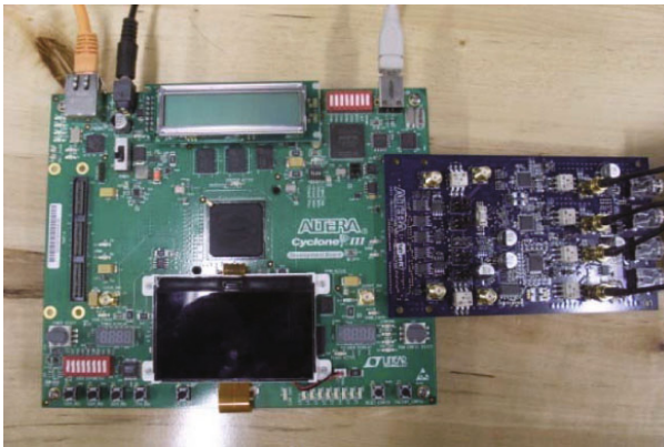
Fig. 4. The snapshot of the prototyping based on the Cyclone III FPGA FPGA development kit
