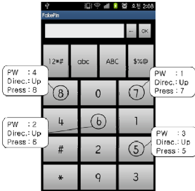
Fig. 1. FakePIN Authentication Phase. The User Presses the Digits <7658> for the Actual Password <1234> in Case of the Direction <Up.>
