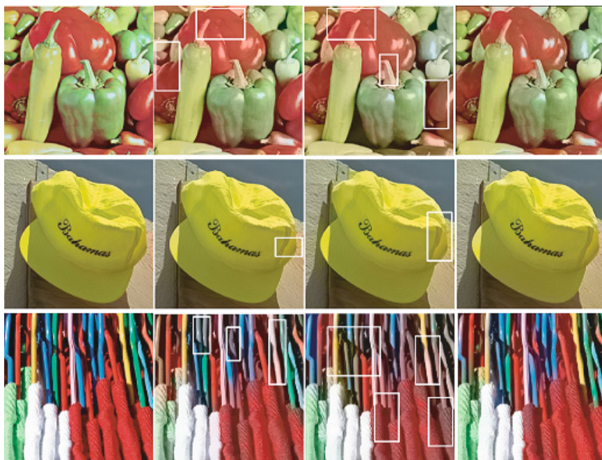
Fig. 3. Comparison of the encoded images of the proposed method and the JPEG standard. Column 1 : Original, Column 2 : Ono's method, Column3 : Cheng's method, Column 4 : Proposed.
