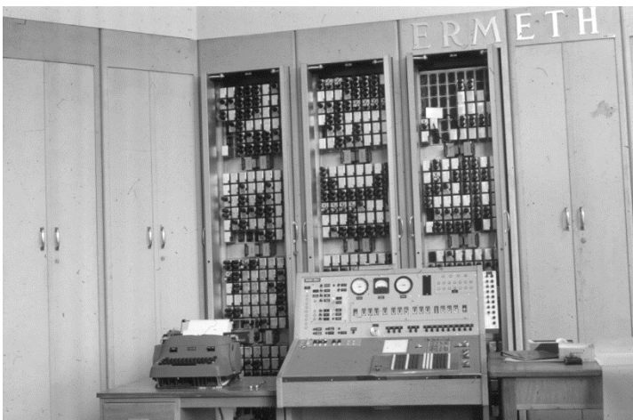
Fig. 7. The first Swiss computer, the stored-program decimal electronic digital ERMETH, ETH Zurich (1956), © Museum für Kommunikation, Berne
