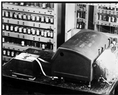
Fig. 10. EDSAC tape reader and teleprinter
