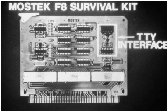
Fig. 3a. Typical single-board 'evaluation kit'
