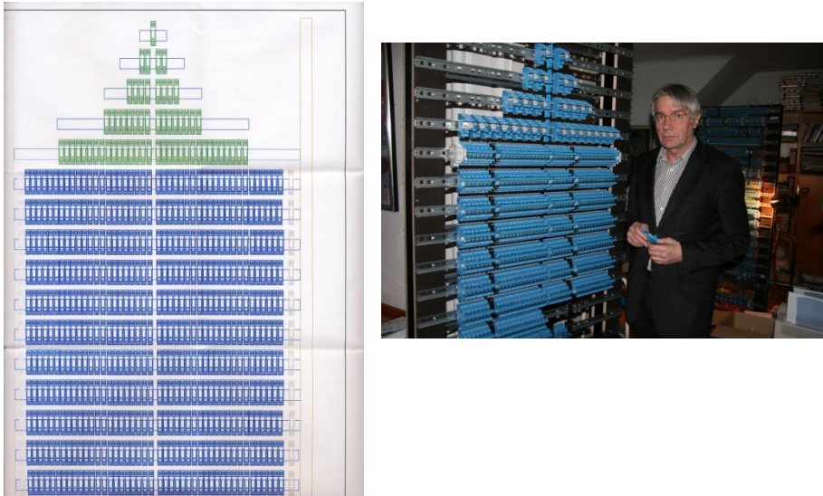
Fig. 9. Left: The design of one memory cupboard. Right: The author building the memory.
