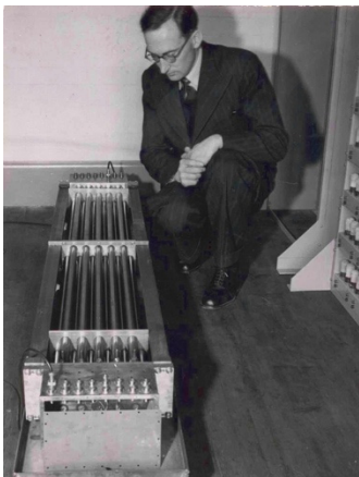
Fig. 8. Wilkes and Mercury Delay Lines
