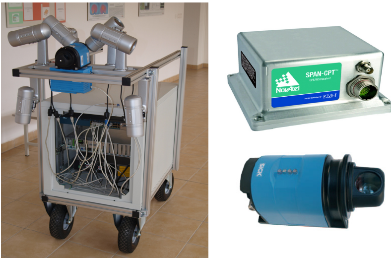
Fig. 1. Photographs of the mobile measurement platform ( left ), the navigation system SPAN-CPT ( right top ) and the laser scanner LD-OEM1000 ( right bottom )
