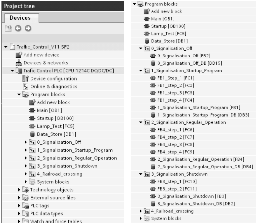
Fig. 3. Program structure in TIA Portal: program blocks structure (to the left) and blocks contents: Functions FC, Function Blocks FB and Data Blocks DB (to the right)
