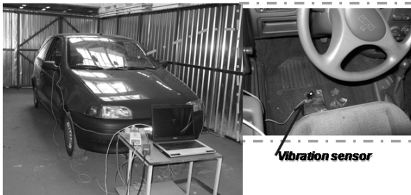
Fig. 2. The object of the research and example of position of vibration sensor
