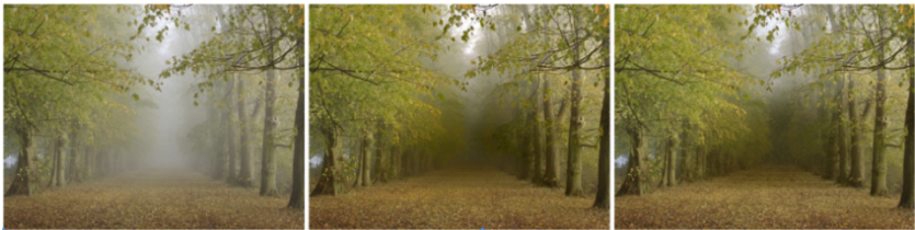
Fig. 1. (a) Input image with haze (b) Result of original HRUDCP (c) Result of modified HRUDCP by introducing guide filter instead of soft matting in step of refining initial transmission. These show that modified HRUDCP is as good as original HRUDCP, and it is the main reason why we introduce the method of guide filter. We get the benefits that we can avoid the need of large memory and decrease the computational complexity of refining initial transmission.
