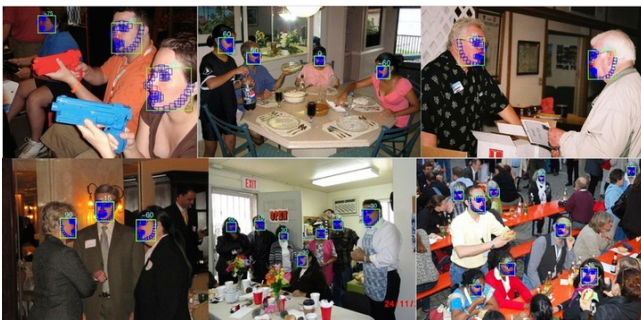
Fig. 4. Results of Ramanan-Zhu algorithm on a "wild" image. The algorithm is able to detect faces in a wide variety of positions and orientations. (Extracted from [3]).
