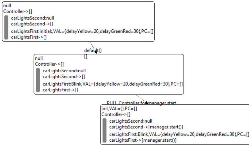
Fig. 3. Exploration step for Controller and \text{AF}(\text{Green} @ \text{carLightsFirst})
