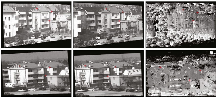
Fig. 8 Experiment for high resolution depth estimation in two successive iterations ( top to bottom ). In each row left camera image, right camera image and corresponding depth map image. Three chosen points (marked with ‘+’) appear to be at different depths in the high resolution depth map
