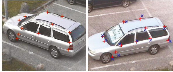
Fig. 6 SIFT 'x' and Chain of Homographies '+' based correspondence between wide baseline stereo images
