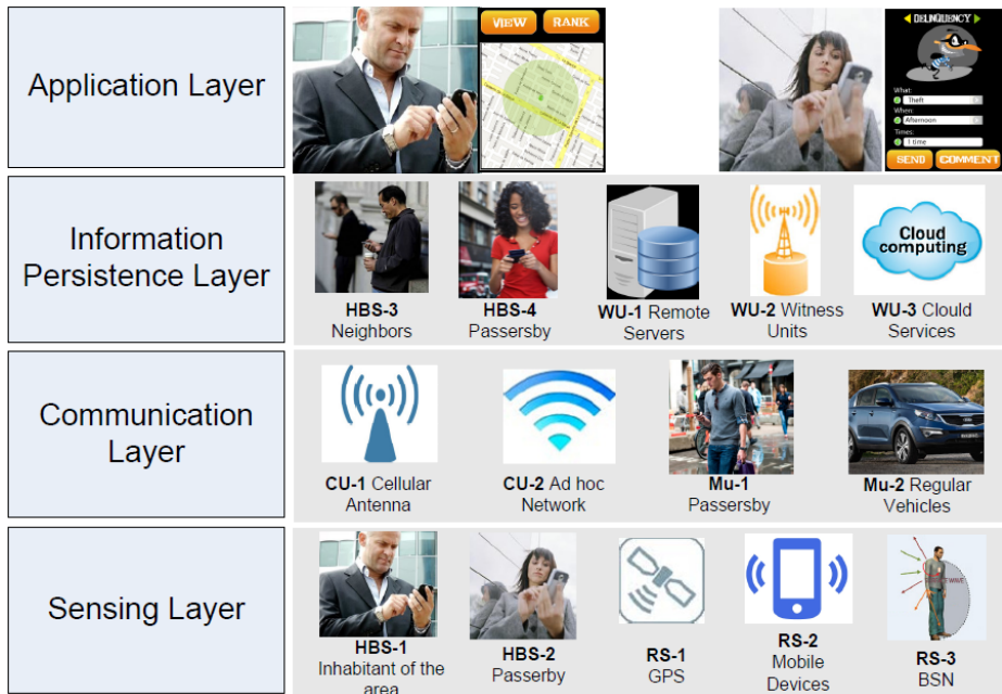
Fig. 1. Layered architecture of a human-centric wireless sensor network
