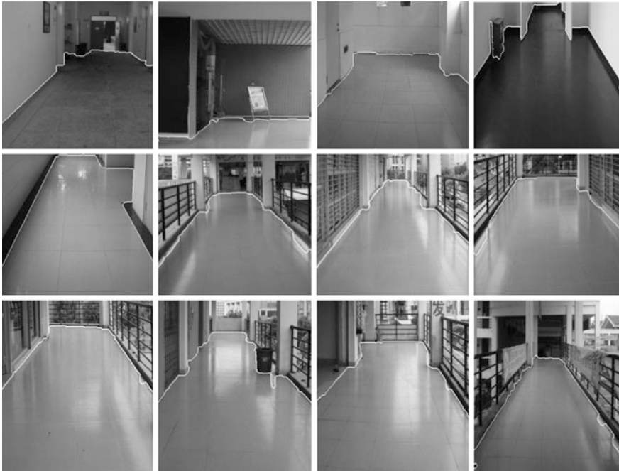
Fig. 27.2 Successful segmentation examples of the corridor floor in our image database which contains corridor pictures with the different material, contours, as well as different building environments
