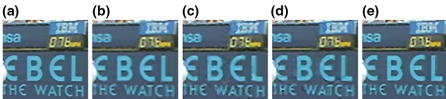
Fig. 26.5 The details of one part of the 88th video frame of the “Stefan” video sequence: a the ground truth; b–e the reconstruction video frames by Bicubic, MSR [11], DSR [12], and the proposed approach, respectively, with MF = 2 \times 2 and p = 3
