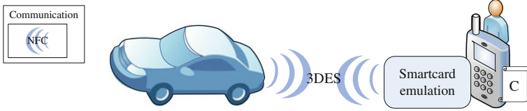
Fig. 4. For executing the granted rights at an NFC object, the smartphone emulates a contactless cryptographic smartcard (here, a Mifare DESFire card). The NFC reader in the door lock of the car detects the presence of the smartphone and initiates the communication. After establishing a secure channel (with 3DES), the credential C is transferred from the phone to the car.
