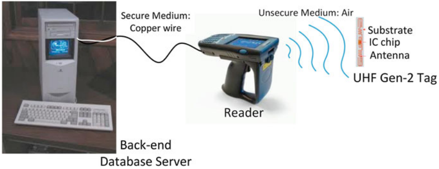
Fig. 1. A typical UHF RFID tag reading scenario
