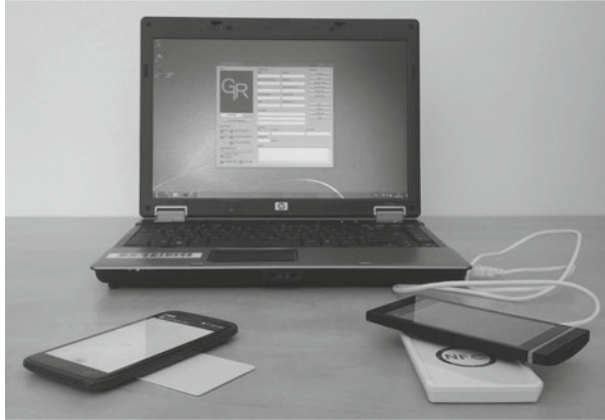
Fig. 8. Off-the-shelf equipment used in the relay attack.
