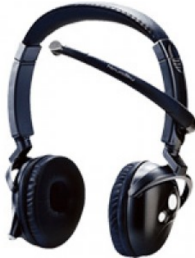
Fig. 1. EEG Headset Used in the Study: Neurosky MindSet
