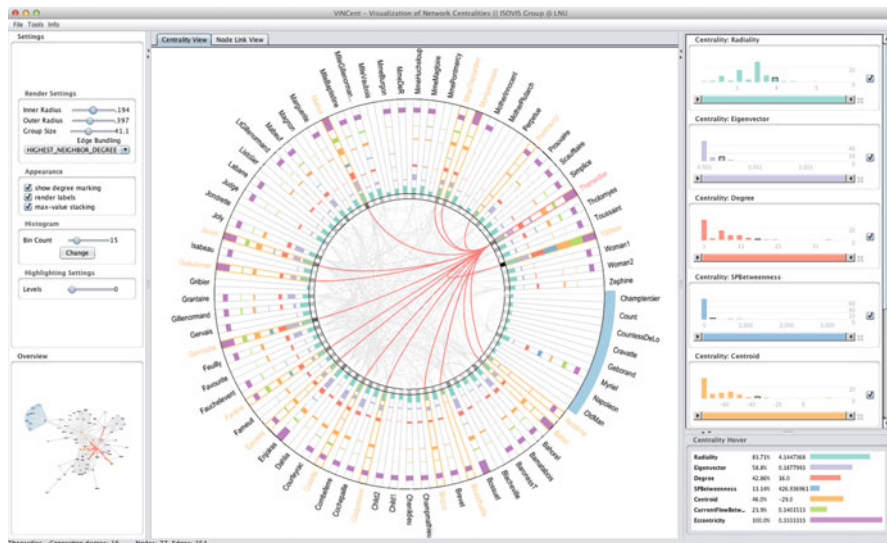
Fig. 7.7 Overview of the ViNCent user interface [150]. The center shows the radial centrality view of the input network. The right side displays the corresponding histograms of the network centralities as well as detailed values of the network centralities for the currently hovered node. Histograms can be used to filter the views. The left panel allows changing the render settings and displays an overview of the respective node-link layout of the network. A node group has been manually selected and is shown as a light-blue stripe along the outer circle in the centrality view as well as in the overview (bottom left) by using a background region of the same color (Color figure online)
