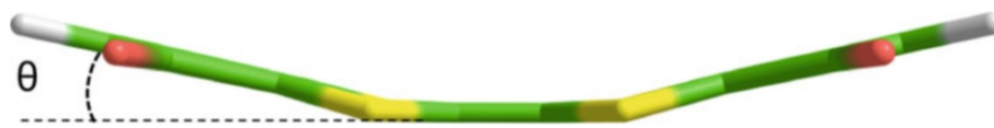
Fig. 2 Minimum-energy structure ( C_{2v} , boat conformation) computed for Q-TTF-Q at the B3LYP/6-31G** level in gas phase. Sulfur and oxygen atoms are in yellow and red, respectively
