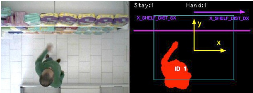
Fig. 2. Example of the water filling algorithm detecting customer with ID 1 together with the shelf line estimated by the depth sensor and the reference system. This second aspect will be better described in section 2.3
