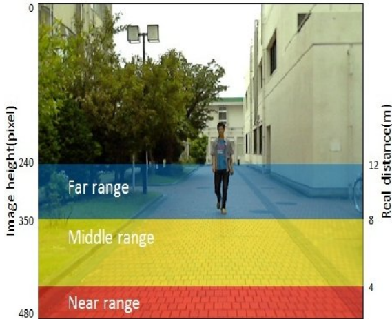
Fig. 5. The relation with distance shown on the camera image
