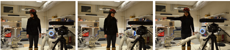
Fig. 3. Data capture session: motion capture makers are placed on the helmet and on the arm
