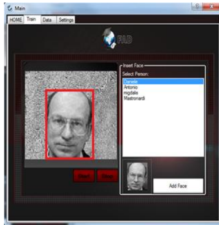
Fig. 2. Enrollment phase with face-detection and face characterization processes
