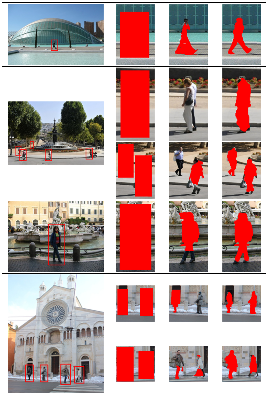
Fig. 2. Visual comparison of the segmentation results. First column contains the original image with the detected people. The other columns show the area to be inpainted using the bounding box, the GrabCut and the proposed approach respectively.
