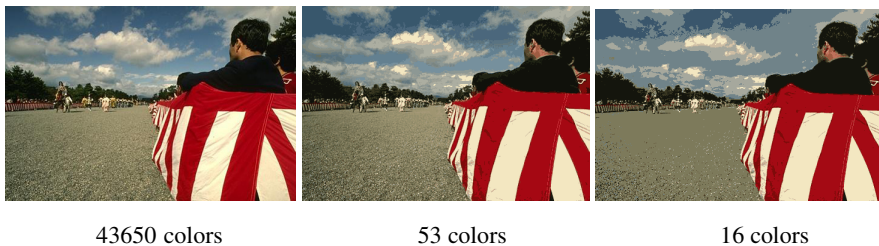
Fig. 1. Input image, left, image resulting after the first phase of CQ, middle, and after the second phase of CQ, right
