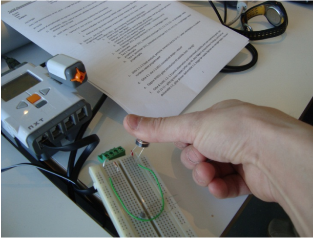
Fig. 11. Testing and calibrating the light sensor
