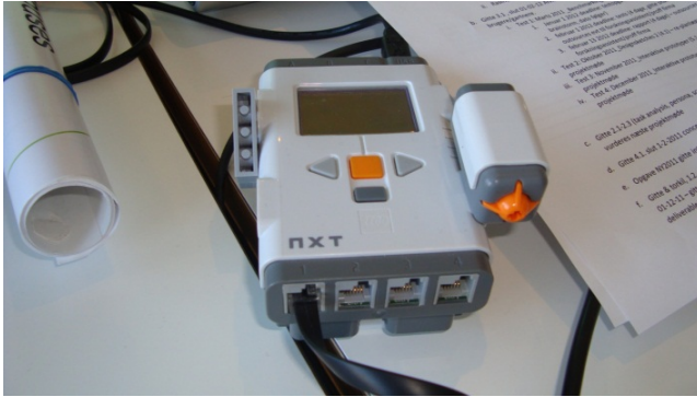
Fig. 5. LegoMindstorms NXT as the platform for prototyping
