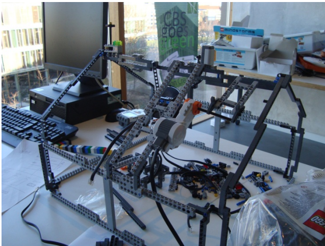
Fig. 6. Prototype 2 - Model of greenhouse
