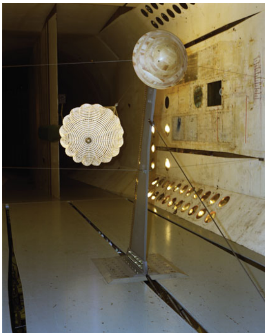
Fig. 18.4 A parachute for the Galileo spacecraft is tested in a wind tunnel at NASA Langley Research Center. Galileo used a conical ribbon, ballistic parachute. Image NASA; GPN-2000-001911 (18 April 1983)
