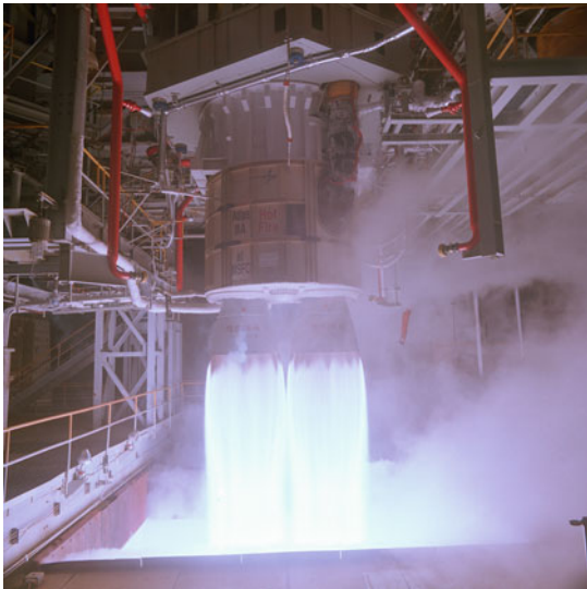
Fig. 11.6 Test firing of the Atlas III propulsion system configured with the Russian-designed RD-180 engine on November 4, 1998 at the Marshall Space Flight Center (MSFC) Advanced Engine Test Facility. The RD-180 is powered by kerosene and liquid oxygen. Image NASA
