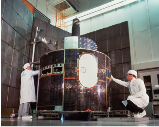
Fig. 12.4 The spin-stabilized Meteosat satellite integration at Aérospatiales Cannes facilities
