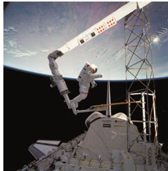
Fig. 19.1 Space shuttle remote manipulator system (SRMS) used as a platform for an astronaut's extravehicular activity in the Shuttle cargo bay. Image NASA/CSA
