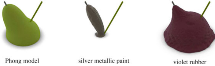
Fig. 6 Simple mathematical models for bidirectional scattering distribution functions (BSDF) f_s(\omega_o, x, \omega) use only a small number of basis functions, like for example the Phong model, and therefore cannot efficiently capture the variety and precision of measured data, like for example the silver metallic paint or the violet rubber. The two cylinders illustrate the direction \omega of incidence from the right and the direction of perfect reflection exiting to the left (Images courtesy Ken Dahm partially using data from [53]).
