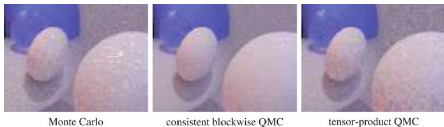
Fig. 4 The images compare three approaches to sampling in light transport simulation computed at an identical number of samples. Obviously the image quality achieved by consistent blockwise quasi-Monte Carlo method is superior to both the tensor product approach and the Monte Carlo method. The quasi-Monte Carlo methods were using the Sobol’ sequence, while the pseudo-random numbers have been generated using the Mersenne Twister.
