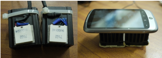
Fig. 1. Peltier modules used to produce thermal icons (left); attached to back of mobile (right)
