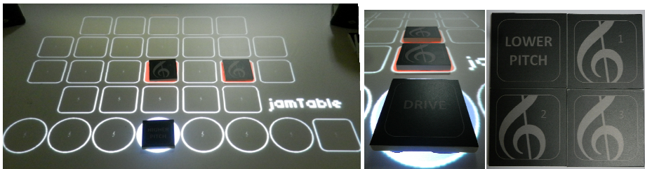
Fig. 2. From left to right: the jamTable’s interface with 24 music tiles (on top), seven control tiles (on the bottom), a record tile (on the bottom right corner), two music tokens playing in sequence (highlighted in red), and a control token (highlighted in blue) applying a higher pitch to the sound being played by the first music token of the sequence; the popular drive effect being applied to two music tokens playing in parallel; and, a closer look at a control token to lower the pitch of a recording, and three music tokens
