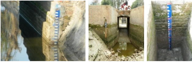
Fig. 1. Examples of manual gauge readout settings for pansal nawisi by Punjab Irrigation Department in Hakra Branch, Bahawalnagar. The water levels are converted to flow using a rating curve derived from channel geometry.
