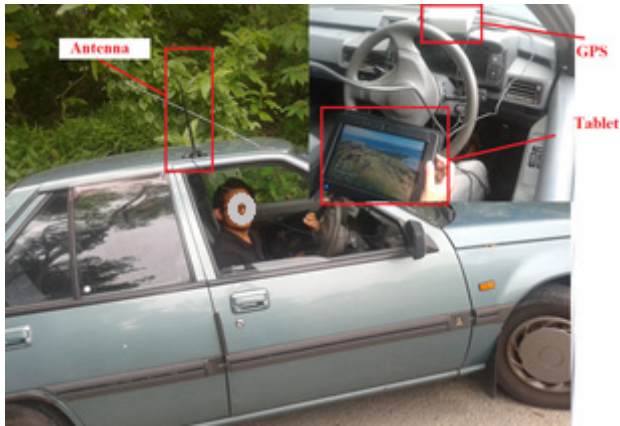
Fig. 6. System equipment on the car to be used for collecting data
