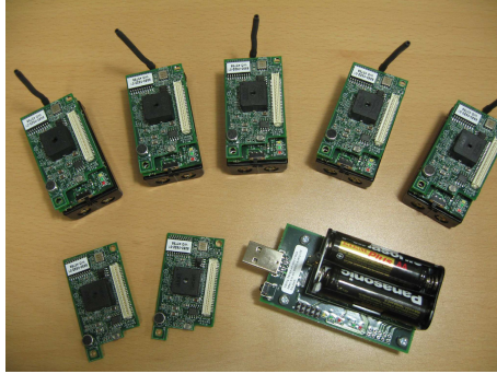
Fig. 5. The wireless sensor devices used to collect both accelerometer and RSS data
