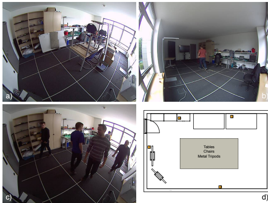
Fig. 7. a) Room with obstacles in the center, b) empty room setup with test subject c) room with 7 persons randomly walking around d) schematic room setup with transmitter coils (orange squares)
