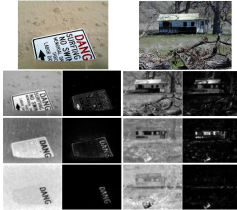
Fig. 5. Sample RGB color images, their respective eigenvector space representations (first, second, and third principal transformations (rows 2–4, columns 1 and 3, top to bottom, respectively), and the respective WTS-based [10] SMCs of each eigenvector space representation (to the right of each transformation image)
