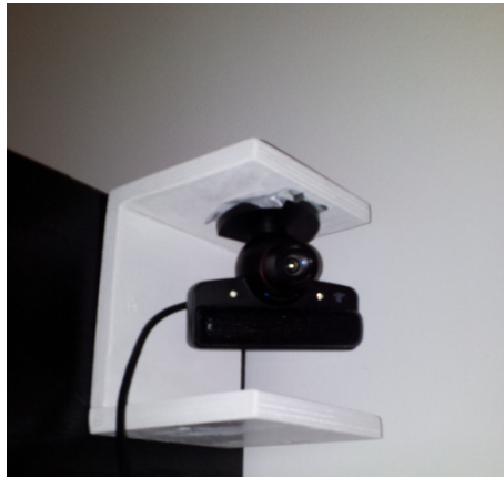
Fig. 9. Custom built stand for Playstation Eye camera
