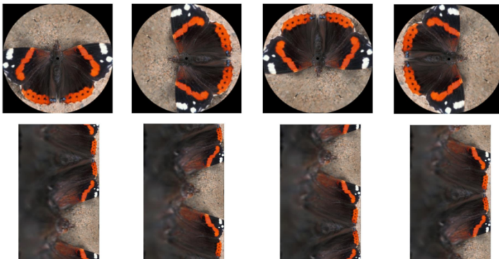
Fig. 3. Top row shows an example image in Cartesian coordinates being rotated successively by \pi/2 degrees in four steps from left to right. Bottom row shows each rotated image in the log-polar domain where the vertical shift is apparent.
