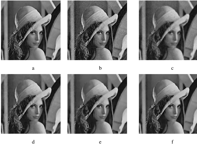
Fig. 4. Lena image restoration: (a) original image, (b) Gaussian degraded image with \sigma = 15 , restoration result using: (c) Tikhonov's algorithm, (d) (ROF) total variation model (e) Multiscale neural network method, (f) Our approach with 400 iteration
