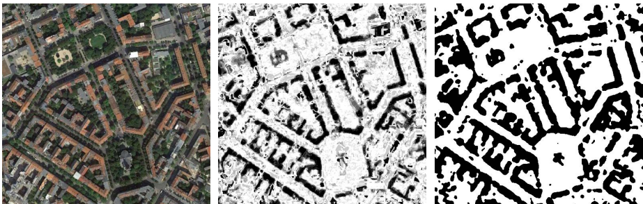
(a) The original testing image. (b) The image after the trainable segmentation process. (c) The image after thresholding.
