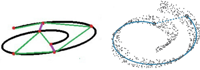
Fig. 1. Left: part of a one dimensional manifold, showing the deficiency of the Euclidian distance (purple edges are shortcut edges), right: Geodesic curve between two points on a manifold (solid line shows the geodesic curve and the dashed line shows the Euclidean curve)
