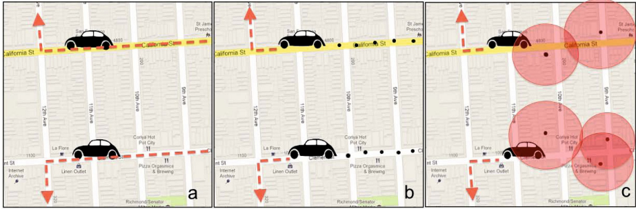
Fig. 1. Two cars running in different streets are going to turn in opposite directions. (a) shows their complete trajectories; (b) and (c) show how they are observed before they turn with GPS and cell-towers data, respectively.
