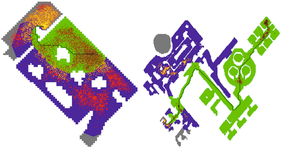
Fig. 5. CH-search on game maps, expanded nodes by Dijkstra (blue), A* (green), CH-Dijkstra (red), bidirectional CH-A* (yellow) and unidirectional CH-A* (black).
