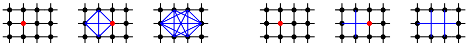
Fig. 1. Illustration of two contraction steps (removal of the red node): On the left without considering ambiguity (or assuming non-uniform costs), on the right with inserting only shortcuts between neighboring nodes if the shortest path via the red node is unique
