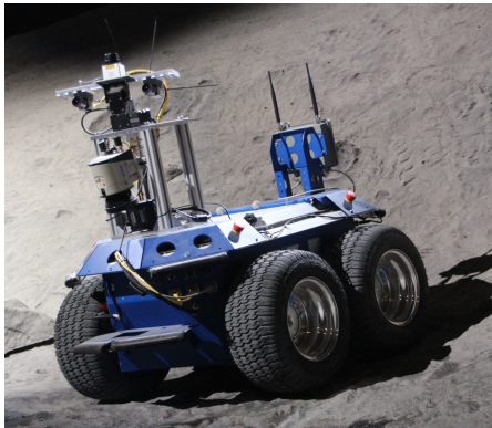
Fig. 3. The robot Seekur Jr. equipped with a couple of sensors
