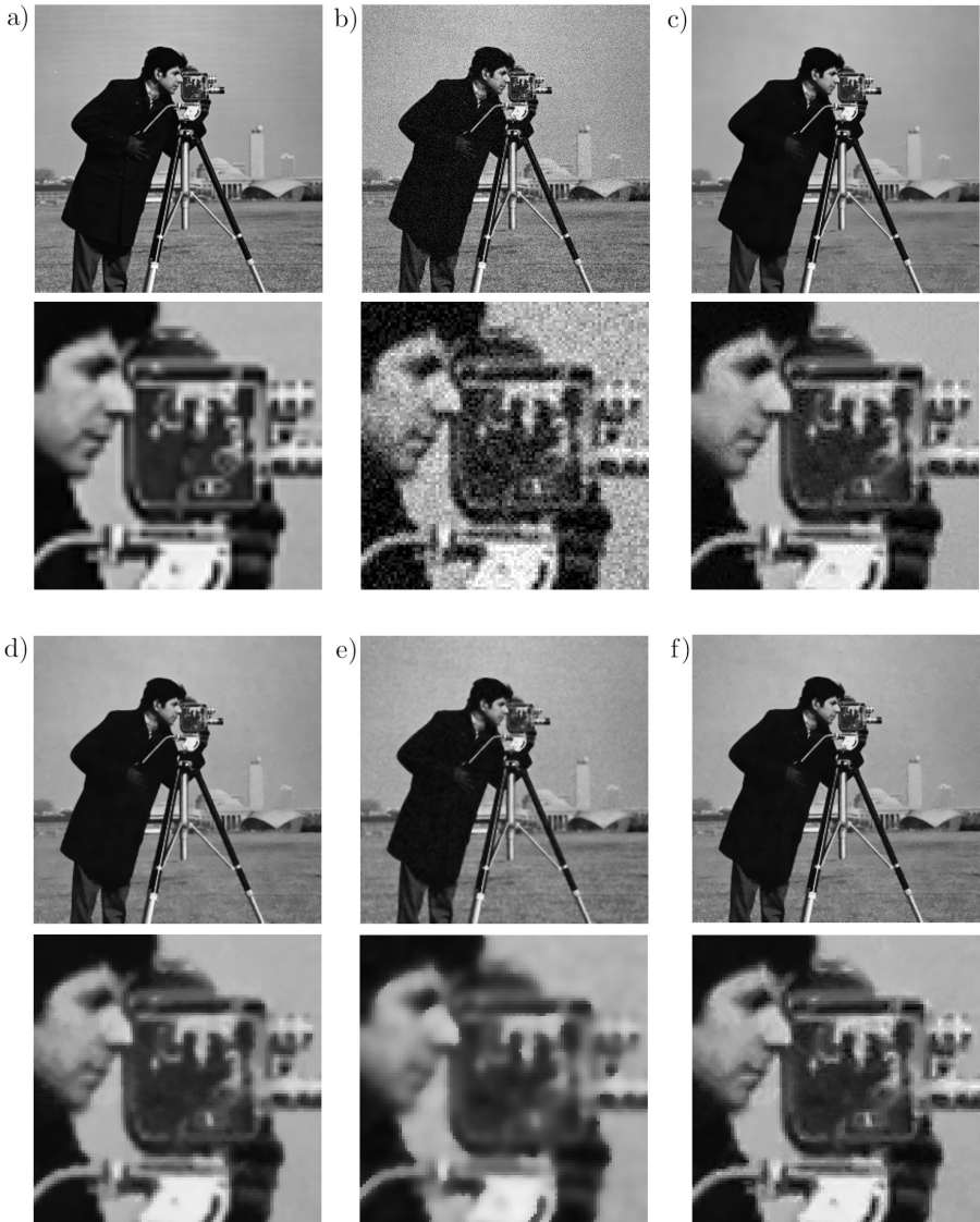
Fig. 4. a) Original image: 512 \times 512 (top) and 96 \times 96 (bottom) b) Noisy image: \rho = 20 c) NL-means: SSIM = 0.9214 d) Stochastic anisotropic diffusion: SSIM = 0.9144 e) Perona-Malik: SSIM = 0.8838 f) New method: SSIM = 0.9196
