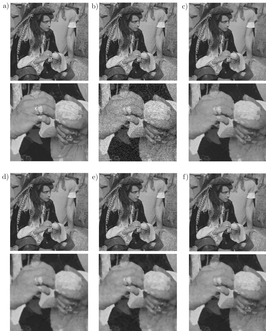
Fig. 3. a) Original image: 512 \times 512 (top) and 128 \times 128 (bottom) b) Noisy image: \rho = 15 c) NL-means: SSIM = 0.9245 d) Stochastic anisotropic diffusion: SSIM = 0.9246 e) Perona-Malik: SSIM = 0.9204 f) New method: SSIM = 0.9257
