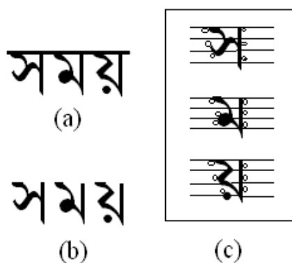
Fig. 2. (a) The Bengali word Somoy with Matra . (b) Somoy after removing Matra , (c) The letters of the word segmented and 3 horizontal partition is done. Also characteristic points have been marked on the left and right contour in each segment for Lateral view based consideration.
