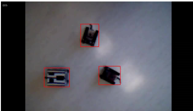
Fig. 7. A frame with tagged targets of the video tracking algorithm
