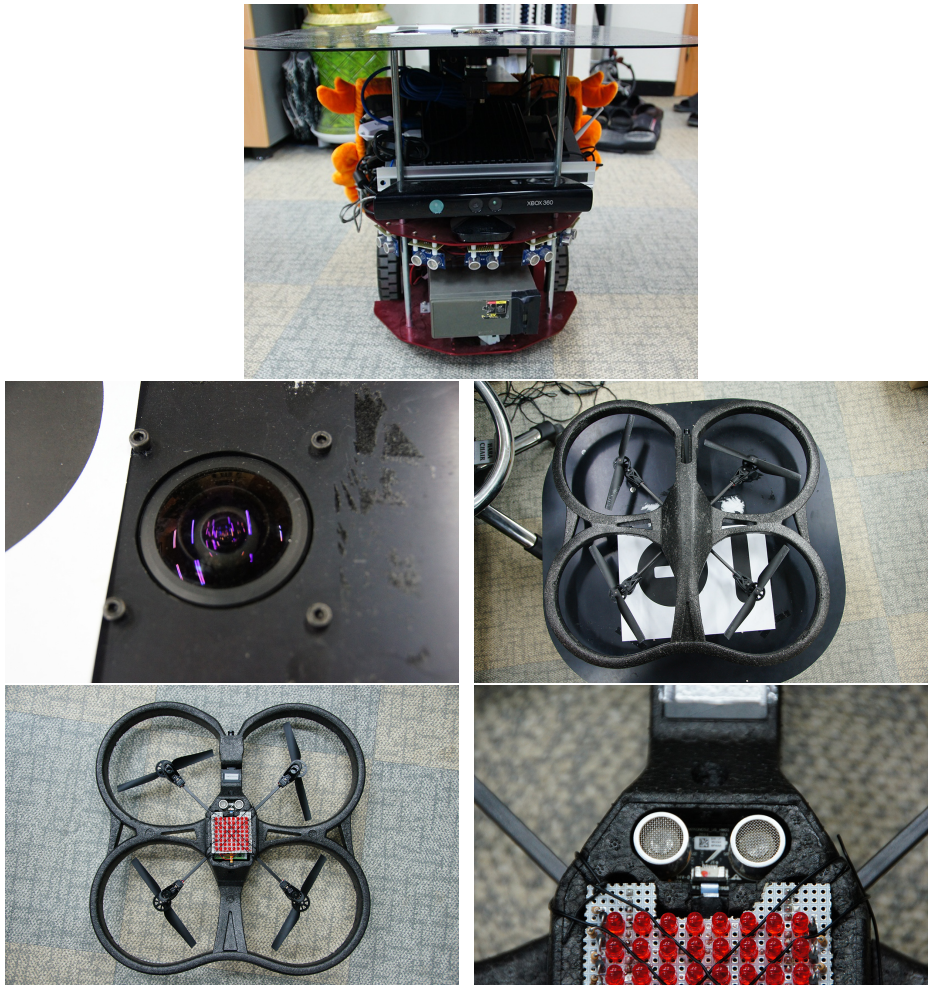
Fig. 6. Integrated Robots: Front view, Fisheye Camera, Landed aerial vehicle, Bottom view, Ultrasonic altitude sensor
