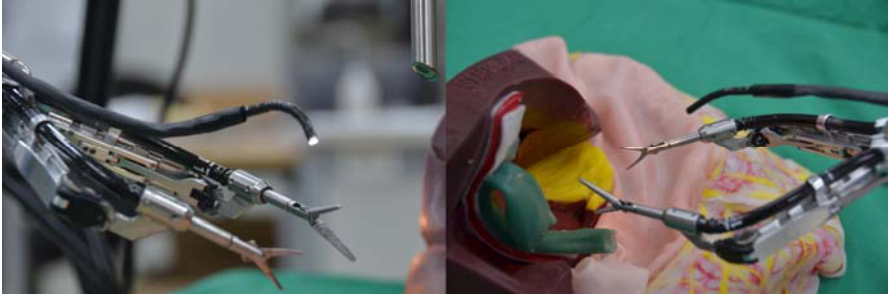
Fig. 5. Final prototype of SILS robot, PLAS
