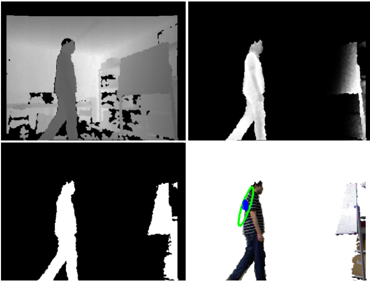
Fig. 3. (a) Depth image from Kinect sensor, (b) depth likelihood image computed from the sample on subject depth value, (c) binary segmentation of (b), (d)
