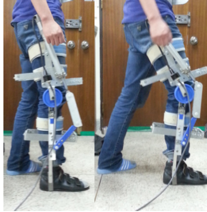
Fig. 1. A robotic knee device with a five-bar linkage for stance control
