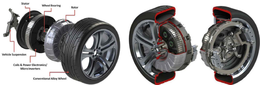
Fig. 1. Conventional in-wheel motor of Protean
