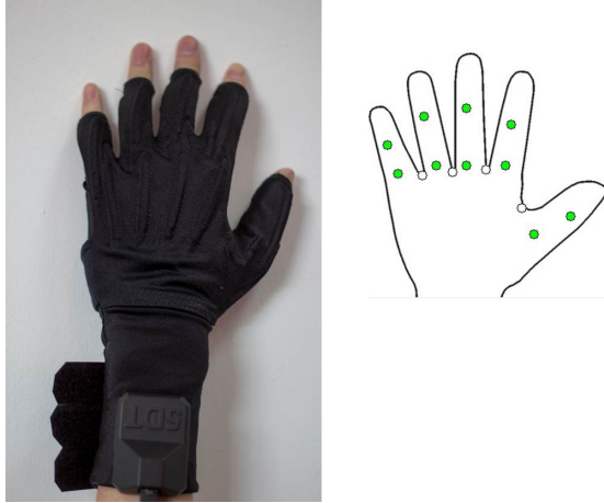
Fig. 2. Finger joint angles acquired by the 5DT Data Glove 14 Ultra from the left arm
