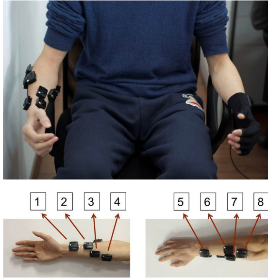
Fig. 1. Sitting position of a subject and position of the EMG electrodes. EMG signals were acquired from the right arm and finger joint angles were recorded from left hand.
