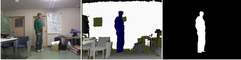
Fig. 7. (a) Color image, (b) depth image with color map, (c) binary human body extraction based on (b)
