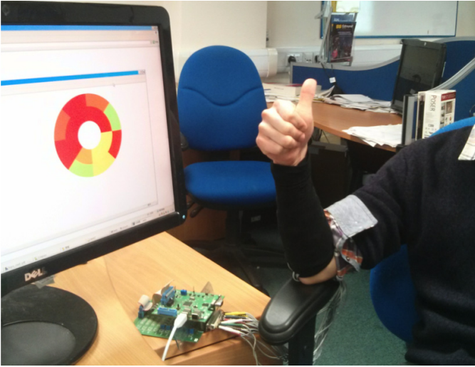
Fig. 6. This picture shows the experimental scene. A subject wears the proposed sEMG electrodes on the right forearm and sits in a chair with the elbow on the armrest. Electrodes are connected to the sEMG device that connects to a PC via a USB port. The software GUI is used to process 16 sEMG signal channels and display it in graphic patterns in real time.
