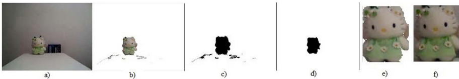
Fig. 1. a) Scenario for image capture, b) Depth segmentation, c) Binary segmented image, d) Filtered segmented image, e) Color segmented image, f) Test image
