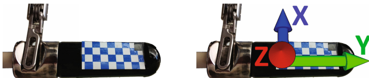
Fig. 1. Left: Picture showing the da Vinci Pro-Grasp tool holding the “pick-up” LUS transducer which has checkerboard markers on it. Right: Same picture as left with addition of 3D coordinate system overlay showing the axes of the LUS transducer marker coordinate system (T). The z axis and the normal of the ultrasound imaging plane are almost parallel.
