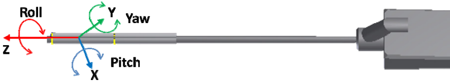
Fig. 3. Convention for defining the endoscope kinematic configuration
