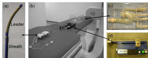
Fig. 4. The experimental setup (b): Hansen Artisan robotic catheter (a), a silicone phantom of the aortic arch (c) and an automatic pullback device (d)
