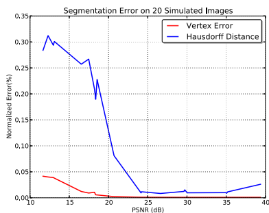
Fig. 3. d_V -PSNR and d_H -PSNR curve. The error is in fraction of the length of the diagonal of the image volume.
