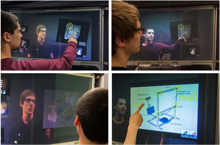
Fig. 3. Gaze direction and pointing gestures are preserved with Face 2 Face. Annotations appear true sided on both client installations.
