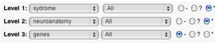
Fig. 6 Using the PathMining query interface to specify a path query. The radio buttons on the right are options for wildcard levels, where “-”, “?” and “*” indicate no wildcard levels, zero or one wildcard levels, and any number of wildcard levels, respectively. This query searches for paths that match the pattern “syndrome → * → neuroanatomy → * → genes”.
