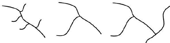
Fig. 9 Illustration of possible structures of long-chain branched polyethylene. Multiple branched comb-like branching ( left ), one 3-arm branch (Y-structure; center ) and two 3-arm branches (H-structure; right )
