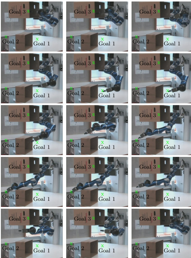
Fig. 7. Real-time motion planning at 500 Hz for a global 3-goals motion planning problem
