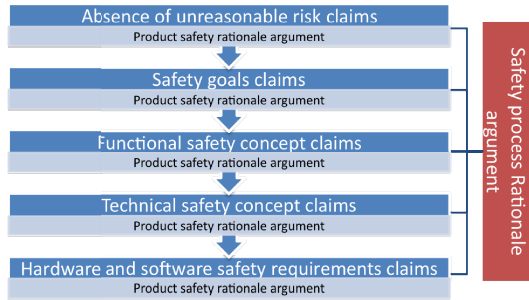
Fig. 1. Implicit ISO 26262 Safety Argument Structure
